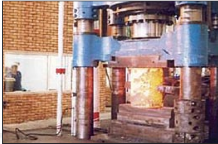
Forge Division: 1800 ton Press – The forging of a bush
